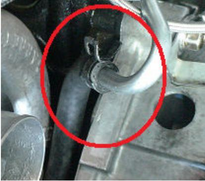
6. Slide the rubber end of the front coolant line assembly (braided line assembly) provided. Slip onto the barb on the waterneck and clamp down as shown in picture.
