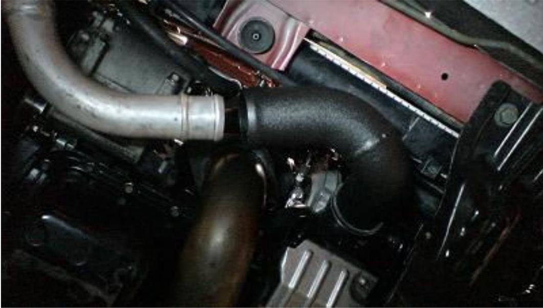
14. Install the 2.5" lower intercooler pipe as shown (join between the compressor discharge pipe and the passenger side of the intercooler).
