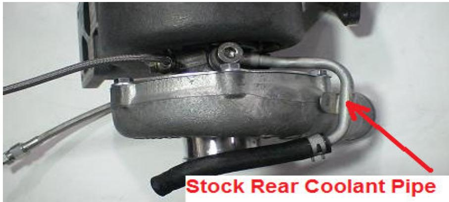
2. Bolt the O2 housing to the turbo using factory gasket and the (5) 10mm studs, nuts and washers provided.
