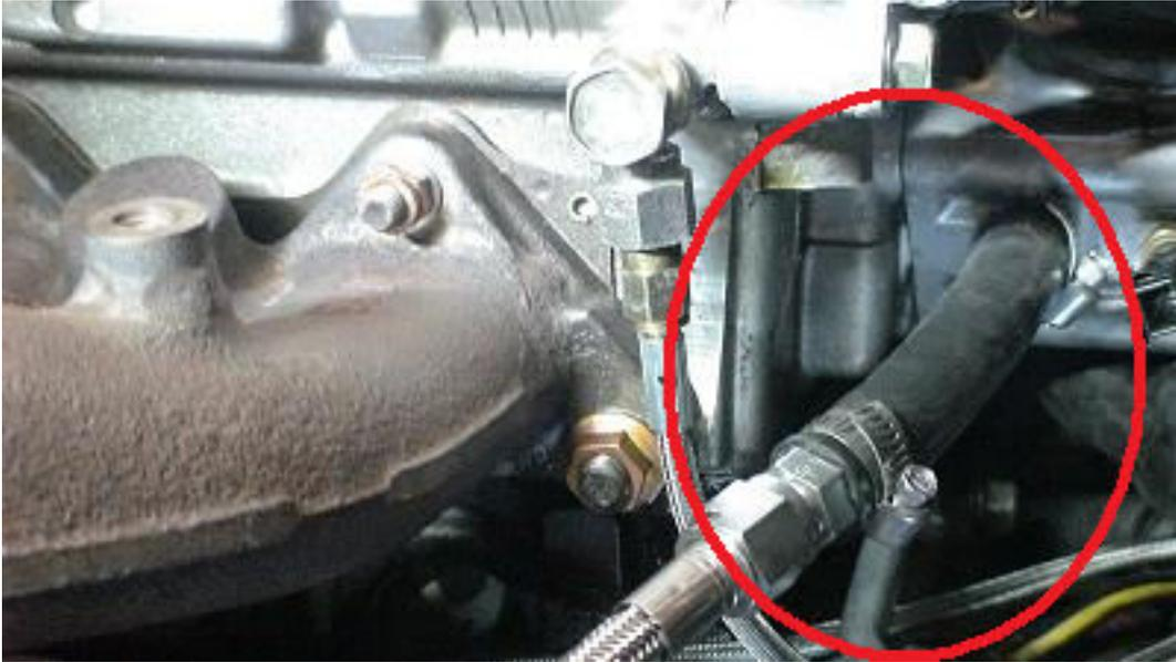
\*\* Note on oil drain install - It is possible to "massage" the factory oil drain tube slightly to get it to line up with the new turbo. If you don't want to take the time, the procedure below is the quickest. It converts the oil drain assembly to a "slip-on" style connection.
