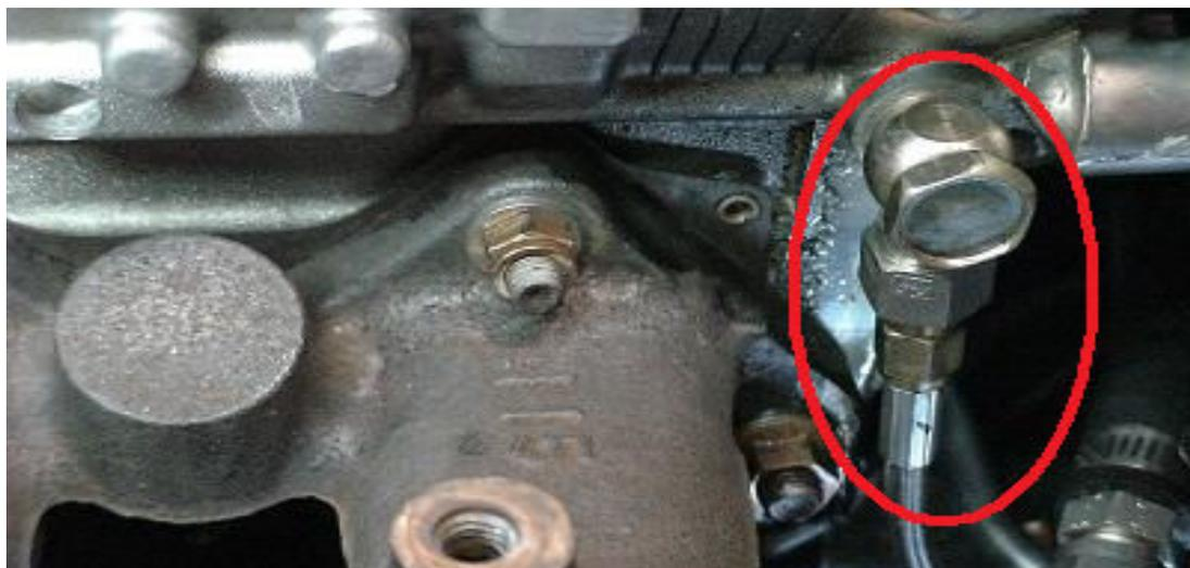
5. Slide rubber end of factory rear coolant hose back into the factory barb and clamp down just like on factory stock turbo.
