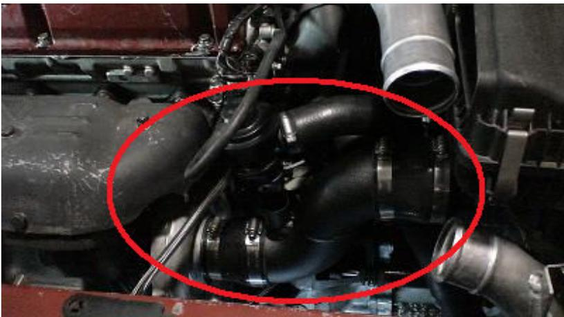
11. Re-install the rubber elbow on the upper intercooler pipe and prepare the radiator hose for re-install of the radiator.
